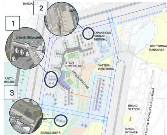
Figure 10: long-term electric aircraft placement options
