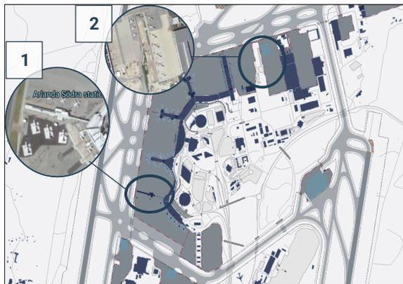
Figure 9: short-term electric aircraft placement options
