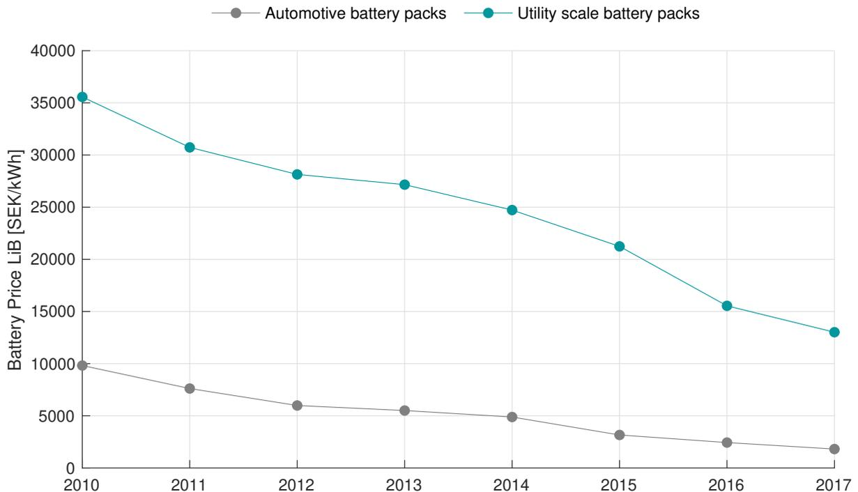
**Figure 5.8:** Evolution of Li-ion battery price from 2010 to 2017 for utility scale and automotive packs.[87]
