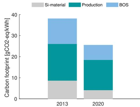
**Figure 8.4:** Carbon footprint for mono-Si PV from 2013 and 2020.[90, 148]
