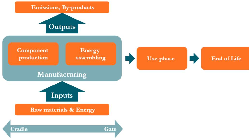
**Figure 8.2:** Stages of life cycle assessment in a battery energy storage system. Edited from original.[141]
