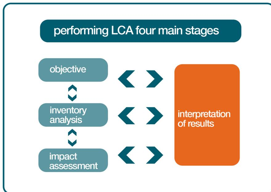
**Figure 8.1:** The four main stages of a life cycle assessment.[140]
