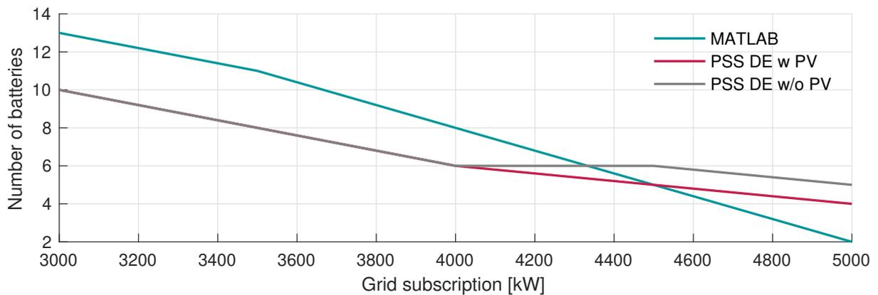
**Figure 10.4:** Total number of batteries and grid subscription needed to avoid blackouts.
