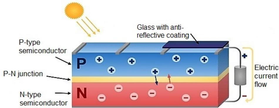
**Figure 6.2:** Electric current flow and semiconductors in a solar cell.[101]
