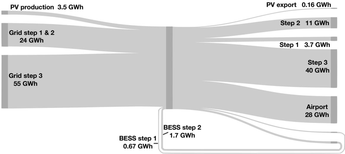
Figure 10.2: Sankey diagram showing total project energy flow from PSS. Edited from original.[80]
