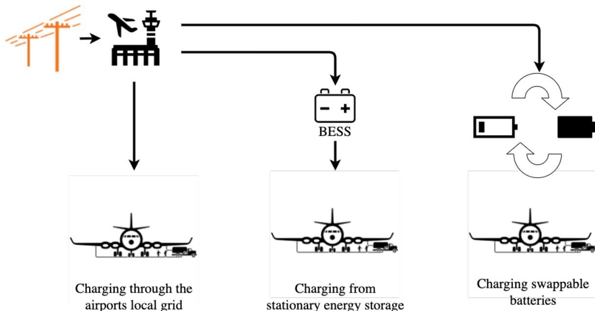
**Figure 3.4:** Three main options for charging electric planes at an airport.[53]
