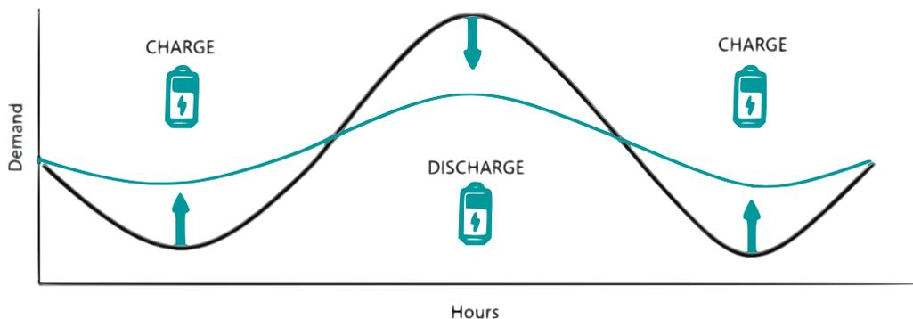
**Figure 4.4:** Battery contributing to peak shaving. Figure made based on theory.[72]
