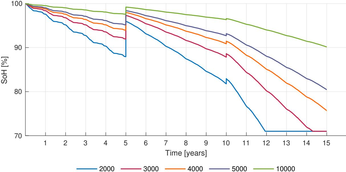
Figure 10.6: Decrease in SoH for BESS in MATLAB for given number of cycles.
