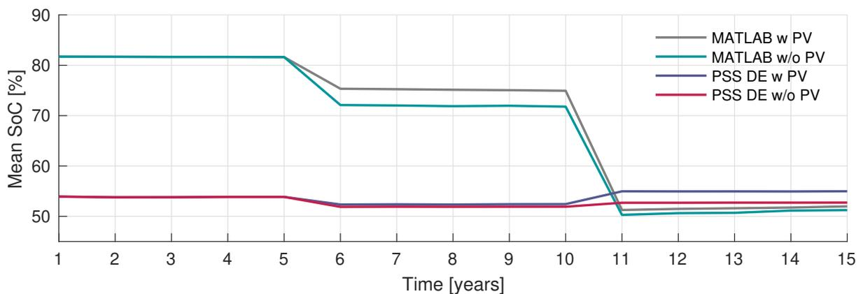
**Figure 10.5:** Mean SoC every year in the simulation with and without PV from MATLAB and PSS.
