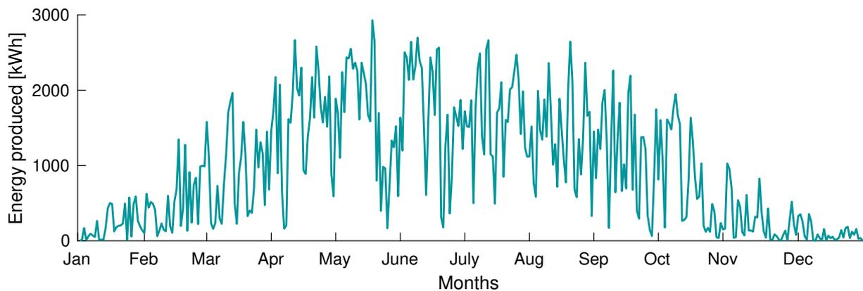
**Figure 9.4:** Daily PV energy output adjusted to snow at Building 90 throughout the year.[100]
