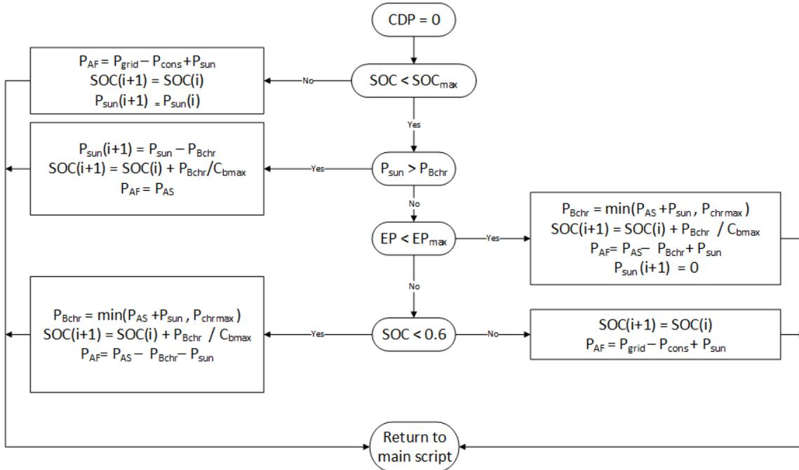
**Figure B.1:** Flow chart for MATLAB simulation when no planes need charging.
