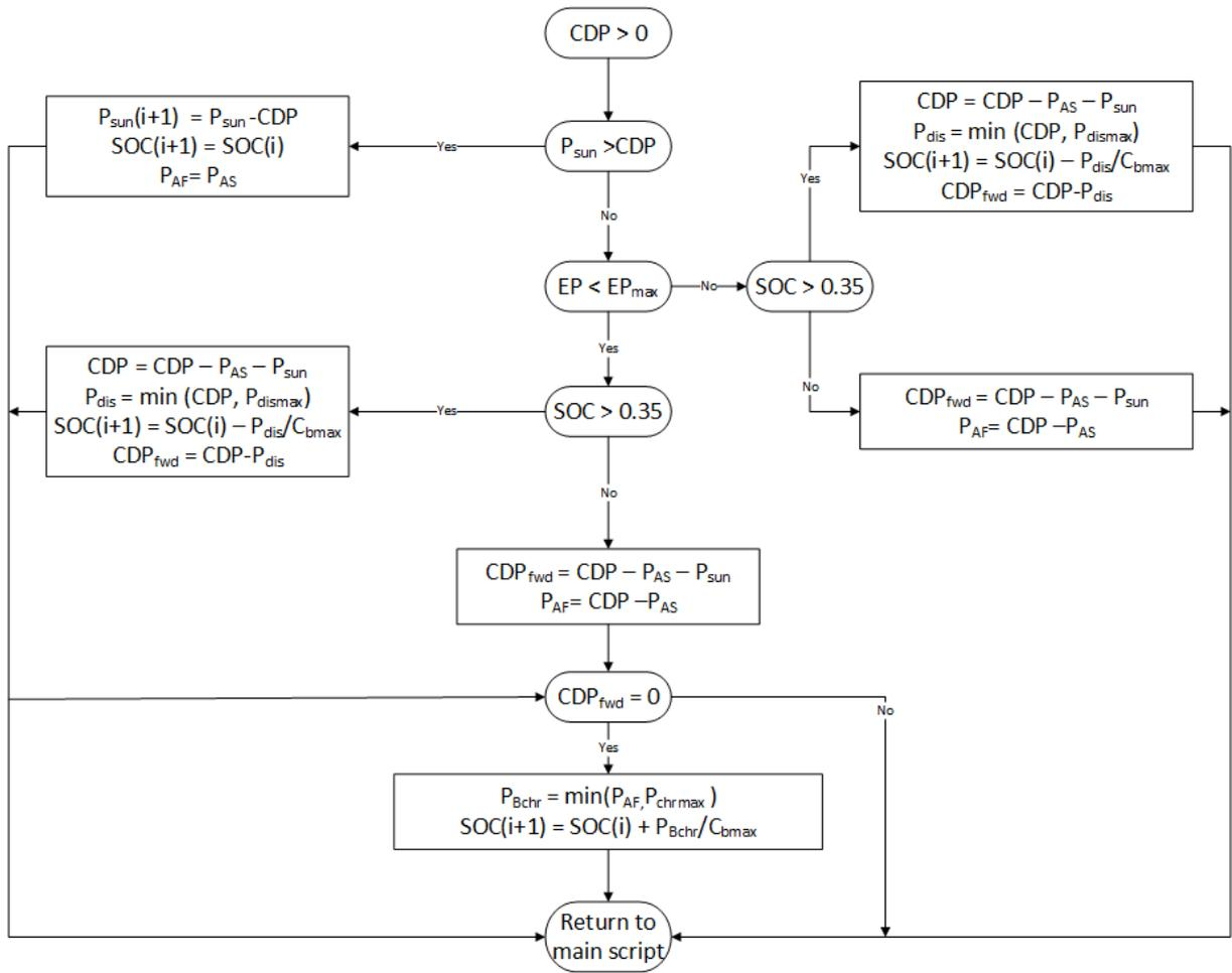
Figure B.2: Flow chart for MATLAB simulation when planes need charging.
