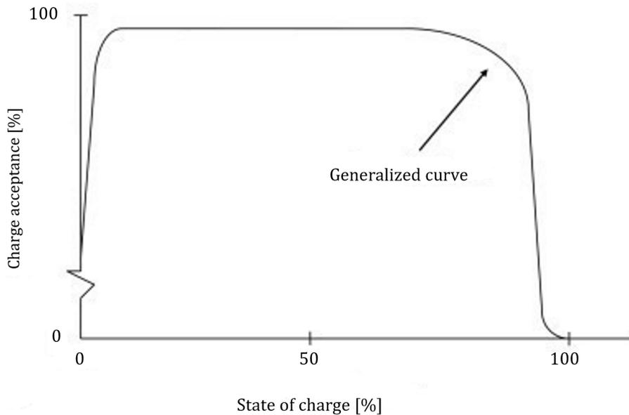
**Figure 5.2:** Generalized curve of effect of SoC upon charge acceptance.[78]
