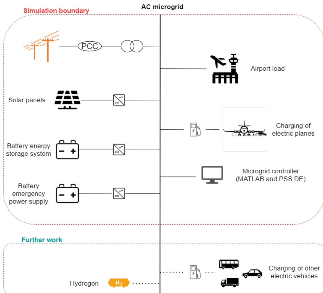
**Figure 9.1:** Schematic diagram of the simulated microgrid system and components in further work.
