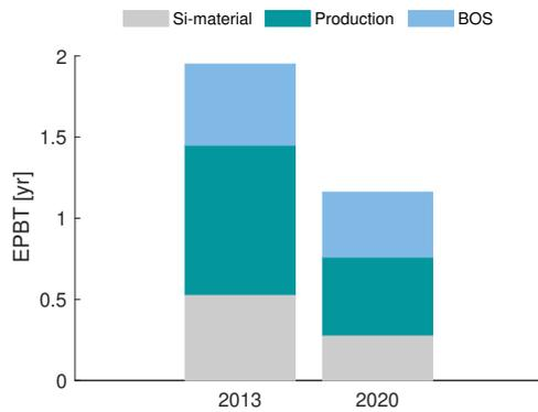
**Figure 8.3:** EPBT for mono-Si PV from 2013 and 2020.[148, 149]
