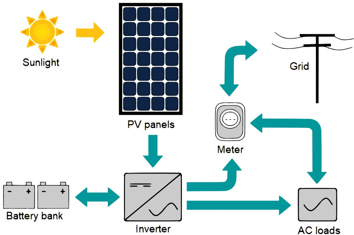
**Figure 6.3:** Components from production to utilization in a PV system.[107]
