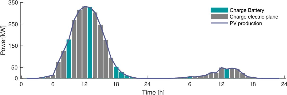
Figure 10.7: Distribution of electricity from PV production for two days in June in step 3.
