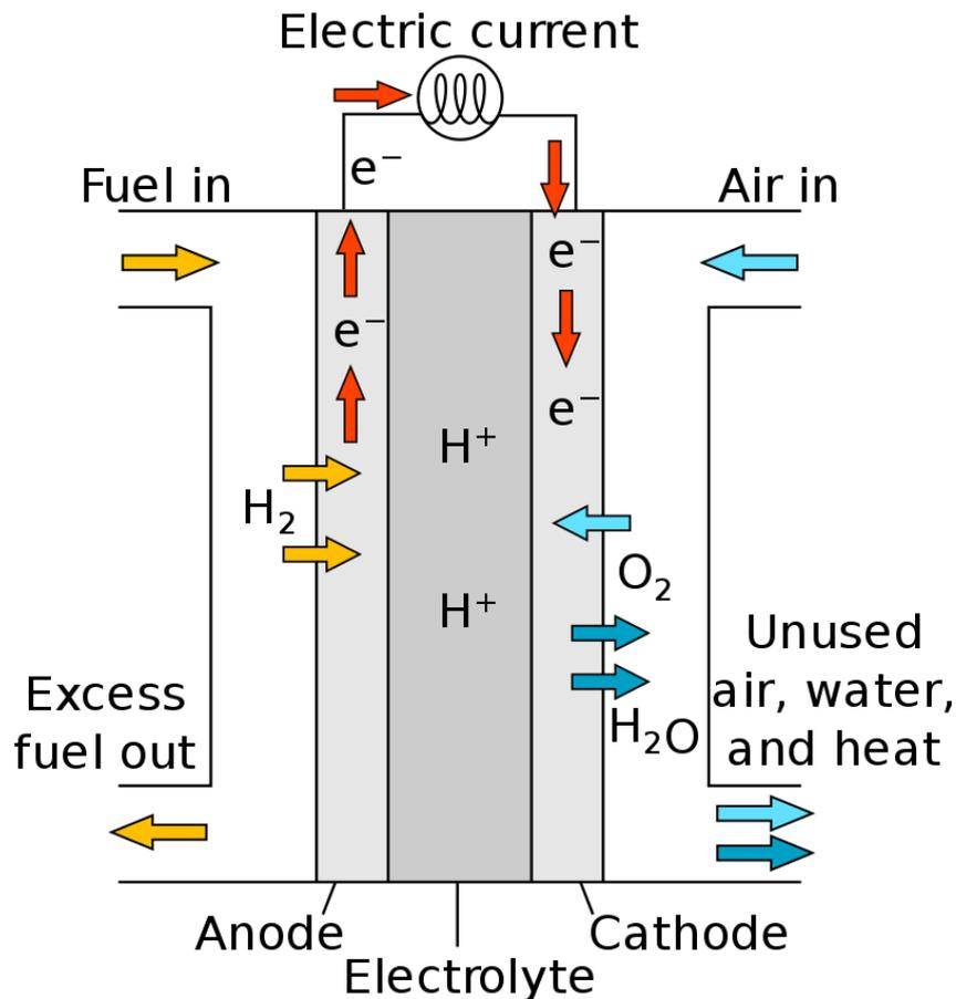
Figure 7.1: Movement of ions in a fuel cell creating electricity.[133]
