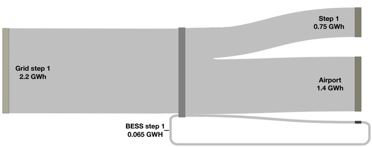
**Figure D.1:** Annual sankey diagram from PSS-DE®Siemens showing step 1. Edited from original.[80]
