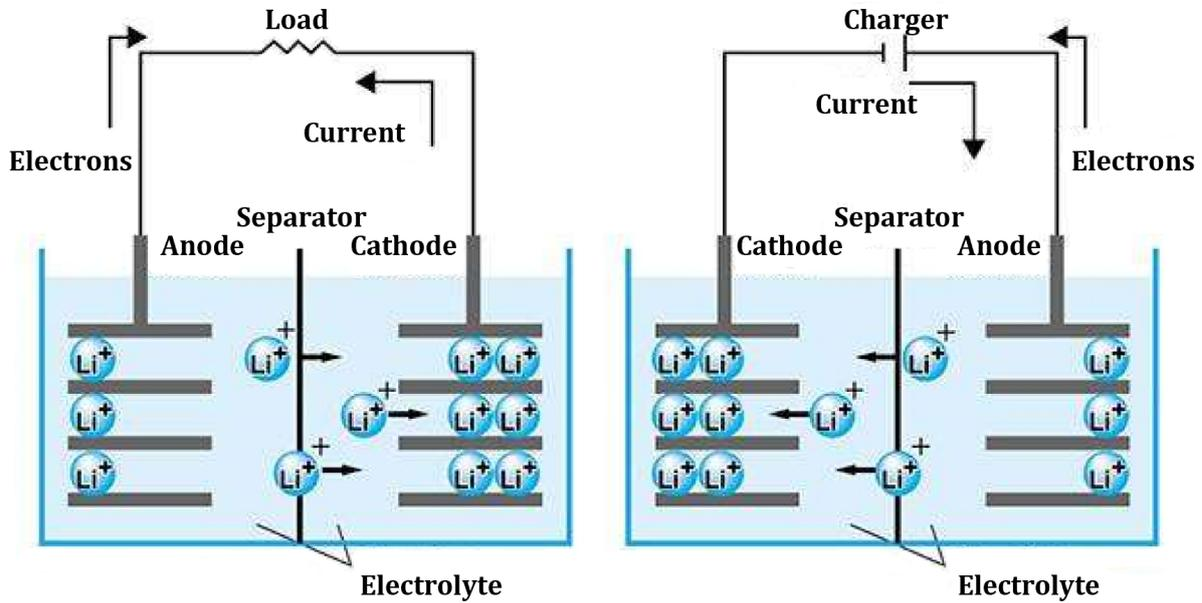
Figure 5.4: Movement of ions in charge and discharge reactions of a lithium-ion battery.[81]
