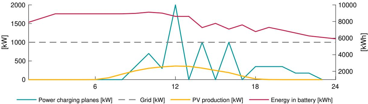
Figure 10.3: Power and energy utilization for 24 hours in April in step 2.
