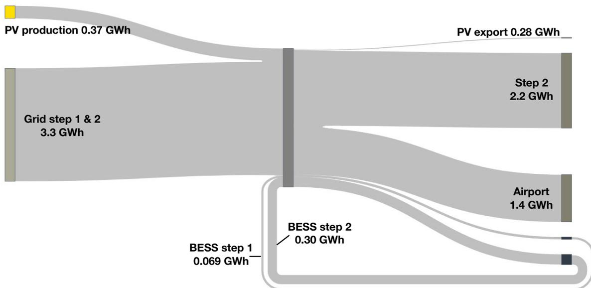
**Figure D.2:** Annual sankey diagram from PSS-DE®Siemens showing step 2. Edited from original.[80]
