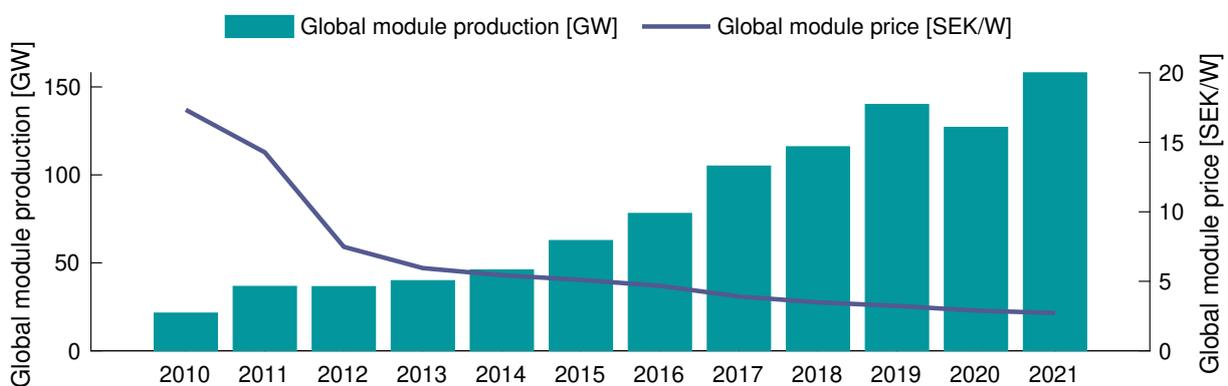
**Figure 6.1:** Development of global PV module price and production from 2010 to 2021.[91–94]
