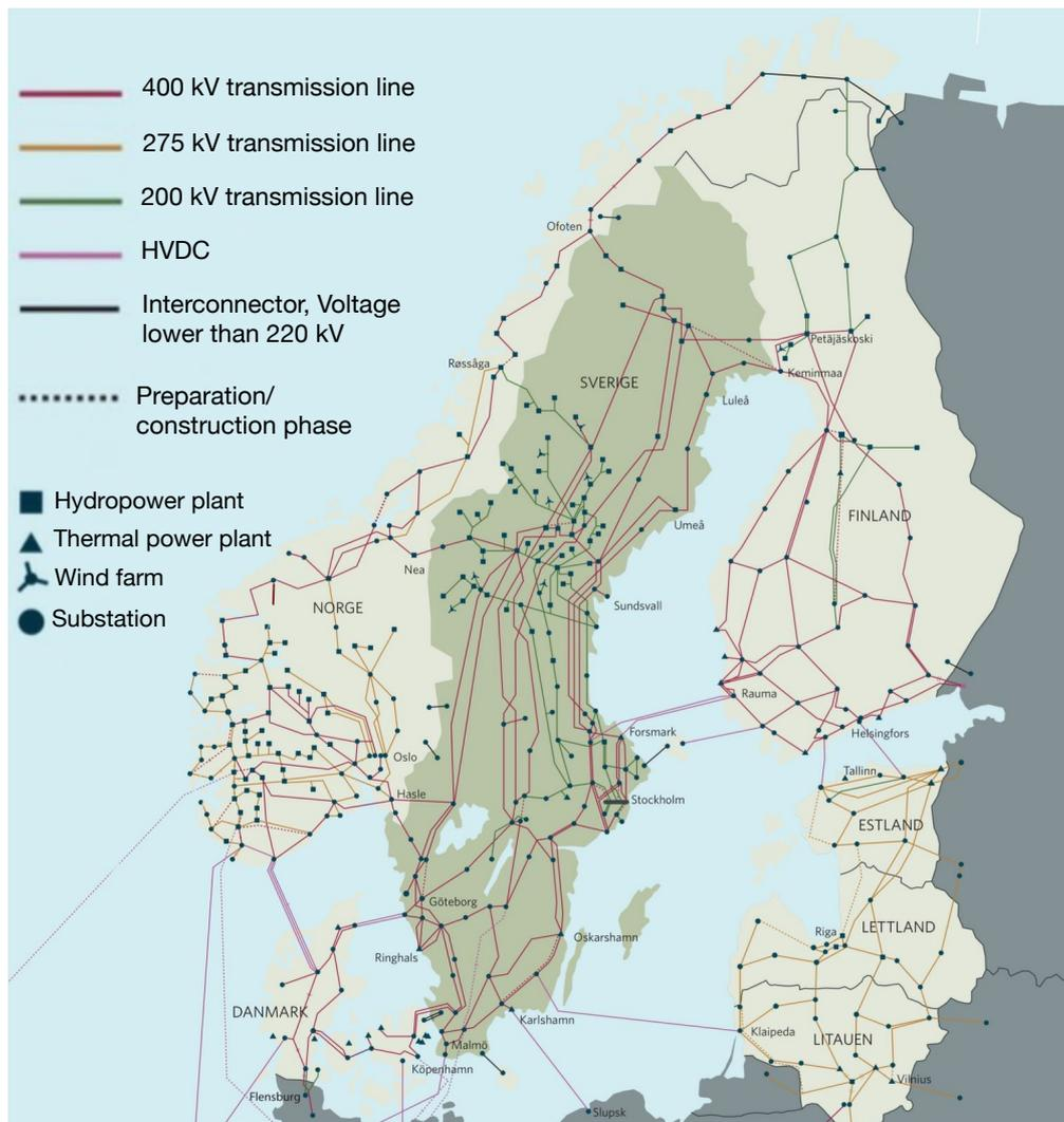
Figure 4.1: The Swedish transmission net with connections to surrounding countries.[58]
