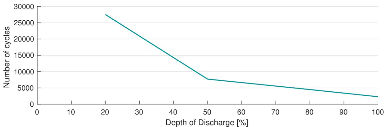
**Figure 5.3:** Cyclic lifetime as a function of average depth of discharge.[80]
