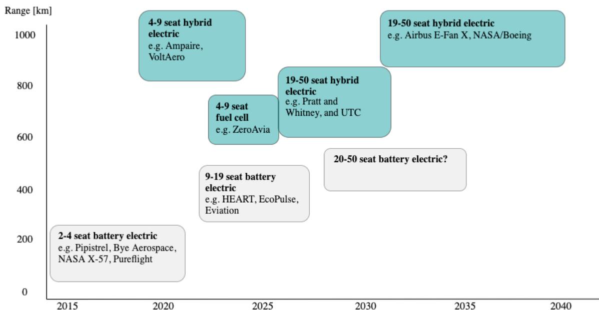
**Figure 3.1:** Timeline for expected technology and range of electric planes. Edited from original.[33]
