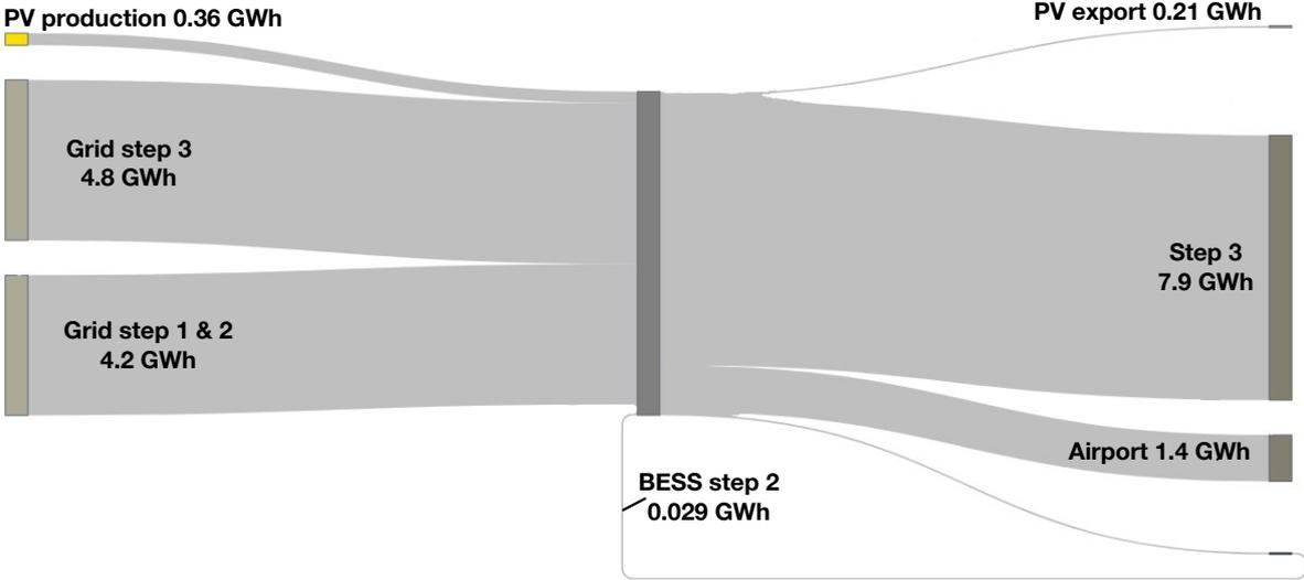
Figure D.3: Annual sankey diagram from PSS-DE®Siemens showing step 3. Edited from original.[80]
